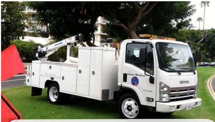
**The ZeroTruck is an all-electric zero emissions medium duty truck based on the Isuzu N series chassis, featuring a low cab forward design and range up to 100 miles.**
